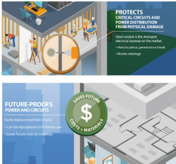
Figure 2. Physical Protection Provided by Steel Conduit. Steel conduit encloses and protects conductors from mechanical damage while allowing future system modifications.
