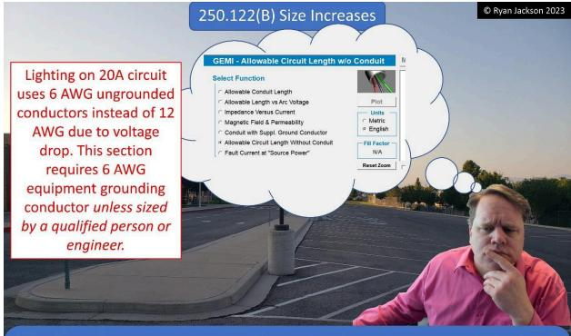
*Ex:* Equipment grounding conductors may be sized by a qualified person if they provide an effective ground-fault current path, as required by 250.4.
