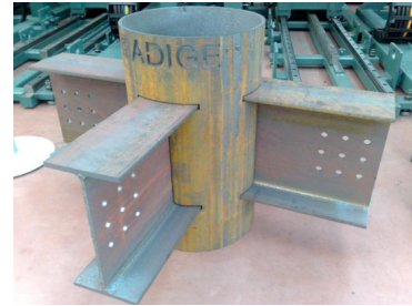
Figure 5: W-shape beams inserted into round HSS column, prior to welding (Adige-Sys SpA)
