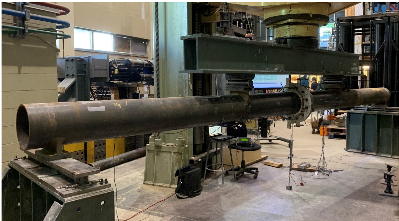
Figure 1: Round HSS end-plate connection tested in flexure
