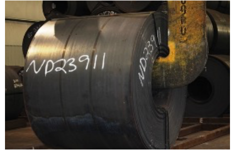
Figure 4: Steel coil used to produce HSS sections
