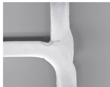
(b) As welded, with penetration to the root
