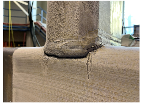
Figure 6: Full-width X-connection loaded to failure, branches in tension, with rupture in the HSS chord
