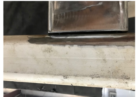
Figure 3: Matched-width T-connection with a large fit-up gap
