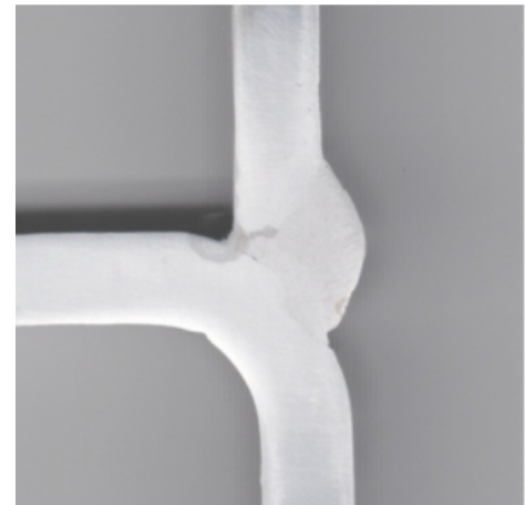
Figure 2: Macro-etched PJP groove weld in a matched-width ( \beta=1.0 ) HSS connection
