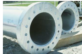
(b) bolted ring-flanges around the HSS
