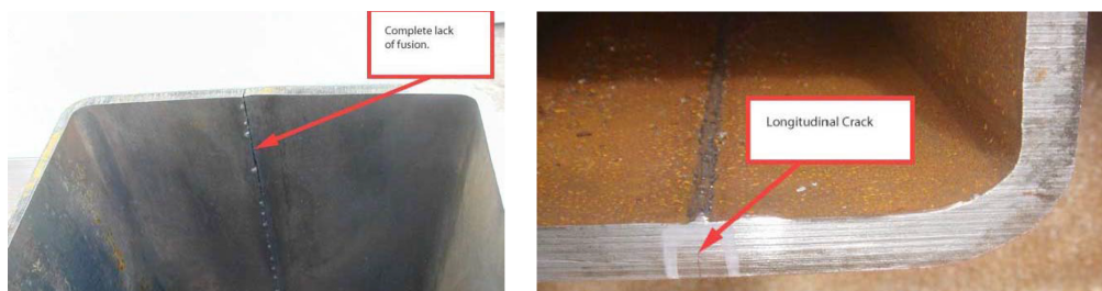
Figure 3: Defective seam welds with imported HSS (Division of the State Architect, California, 2007)
