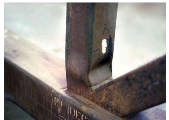
Figure 4: Compression-loaded branch local yielding failure
