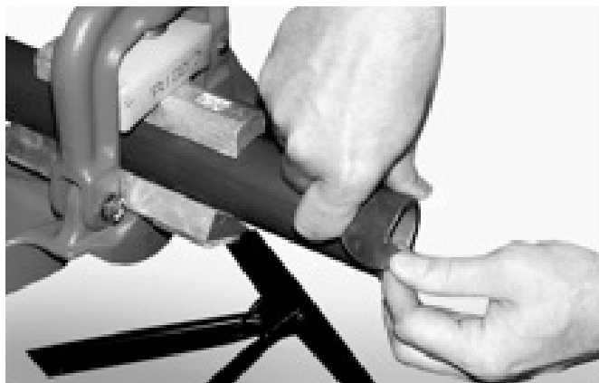
Figure 16: Utility knife used to apply "pencil-cuts" to PVC coating to allow the conduit easier entrance into the cutting die.
