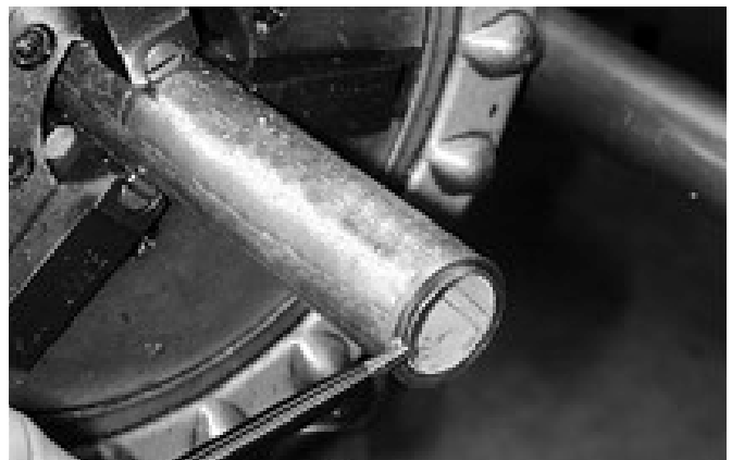
Figure 6: The roll cutter will leave a burr on the inside diameter of the conduit. The burr must be removed to ensure that the wire insulation will not be damaged during pulling.
