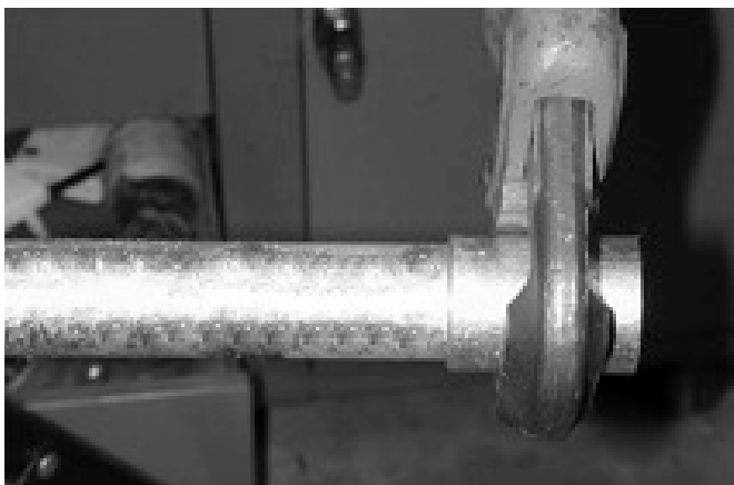
Figure 13: The coupling must be assembled wrench tight.
