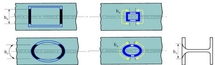
Figure 3: Effective width model for branch local yielding (Wardenier et al. 2010)
