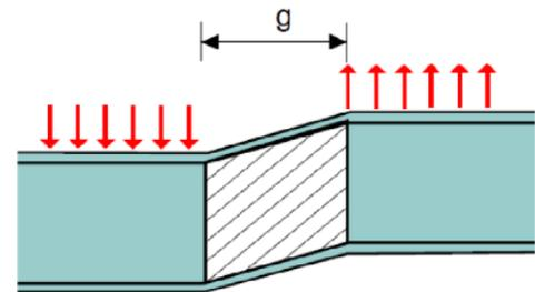
Figure 5: Shear failure in the chord gap region of a K-connection
