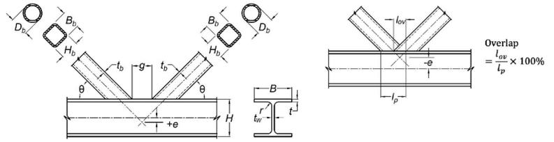
Figure 1: Gapped and overlapped K-connections between HSS branches and I-shaped chord members
