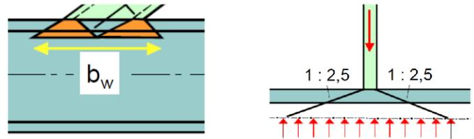
Figure 4: Analytical model for chord web yielding (Wardenier et al., 2010)
