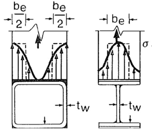
Figure 2: Distribution of stress in the transverse wall of an axially loaded HSS branch, welded to an HSS chord member versus an I-section chord member (Davies and Packer, 1982)
