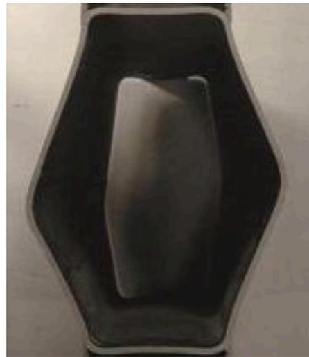
Figure 5: Buckling of HSS side walls under transverse compression
