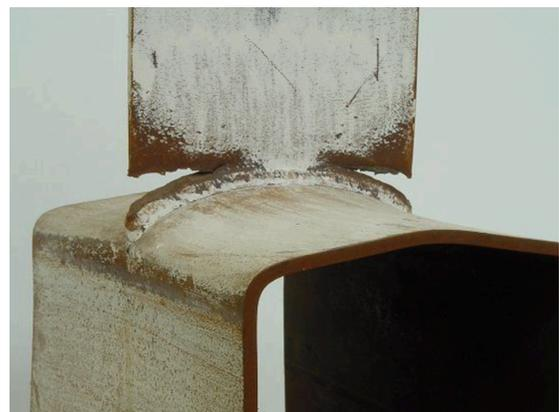
Figure 2: A heavily welded, tension-loaded, transverse branch plate connection (with  $B=1.0$  and high  $\beta/t$ ) demonstrating local failure of the branch plate. The parts of the plate width that are effective are illustrated by the two outer brown regions where the white-wash has flaked off.
