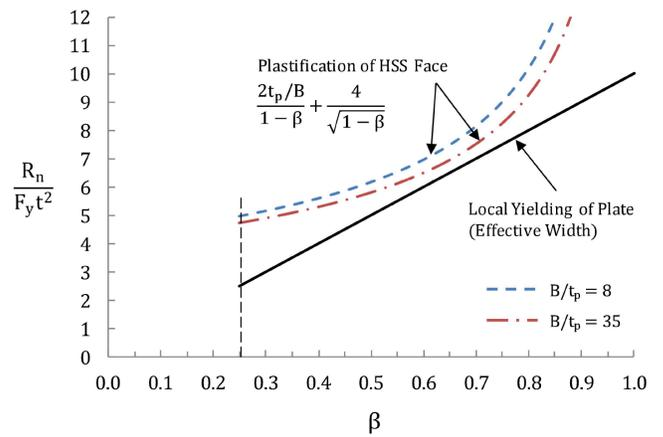
Figure 3: Interaction between *Plastification of the HSS face* and *Local yielding of the branch plate*, for transverse plate-to-rectangular HSS connections
