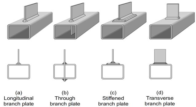
Figure 1: Types of plate-to-HSS connections
