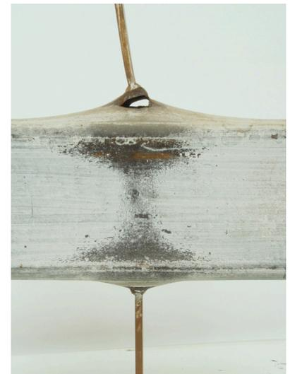
Figure 4: A tension-loaded, transverse branch plate connection exhibiting three failure mechanisms: (i) *Plastification of the HSS face*; (ii) *Punching shear of the HSS connecting face*; (iii) *Local yielding of HSS side walls*
