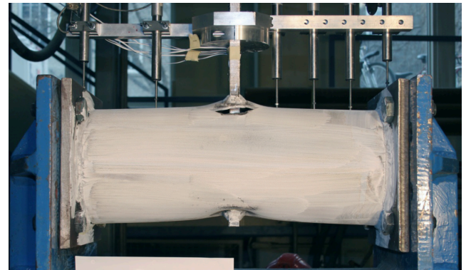
Figure 2: Typical through plate-to-round HSS connection laboratory testing arrangement
