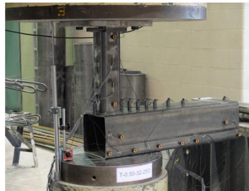
Figure 3: Typical test set-up for HSS-to-HSS end connections
