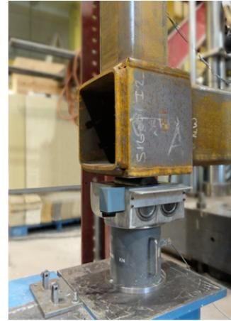
Figure 1: HSS connection near the end of an open chord, with the chord stiffened
