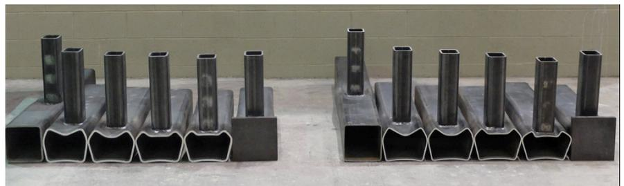
Figure 4: Family photo of all connection specimens, after testing. (Control specimens, with the branch remote from the chord end, are at the left of each group; end-capped specimens are at the right side).
