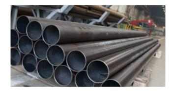
Beyond 20" OD – If your project requires members that exceed what is currently produced in A500, there is piping produced for other industries that can be used in structural applications with caution. Most commonly, products that meet specifications such as API 5L for the oil and gas industries can be procured.
