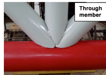
Figure 6: Preferred overlapping sequence
