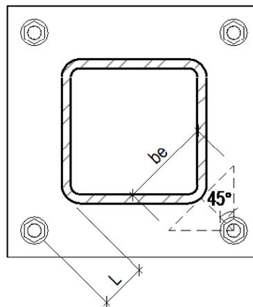
Figure 3 – Typical HSS anchor bolt locations, failure plane and effective widths
