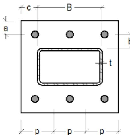
Figure 4 – Alternate anchor bolt layout
