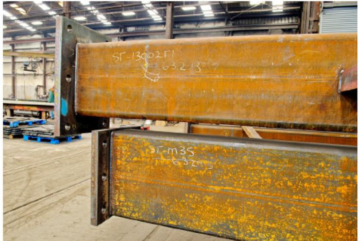
Figure 1 – HSS base plates with 2 different anchor bolt configurations
