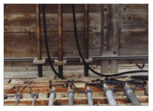
**Photo 8.** Ten runs of RMC, IMC, and EMT metric designator sizes 16 (1/2 trade size) through 78 (3 trade size) connected to the transformer for high current and low current tests.
