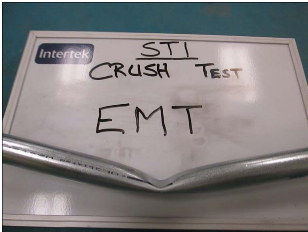
Figure 12. After Crushing Test
