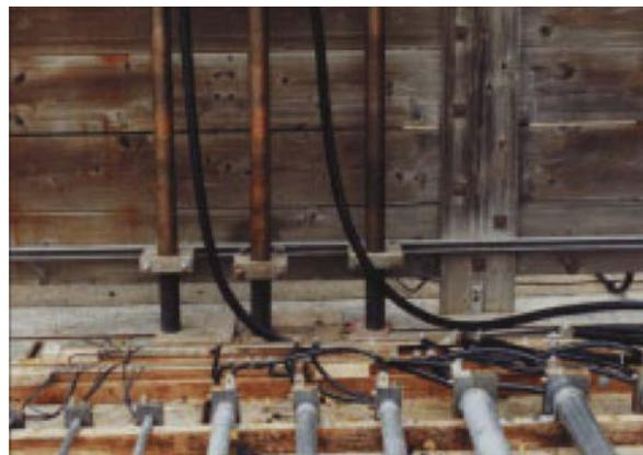
Photo 8. Ten runs of RMC, IMC, and EMT metric designator sizes 16 (1/2 trade size) through 78 (3 trade size) connected to the transformer for high current and low current tests.
