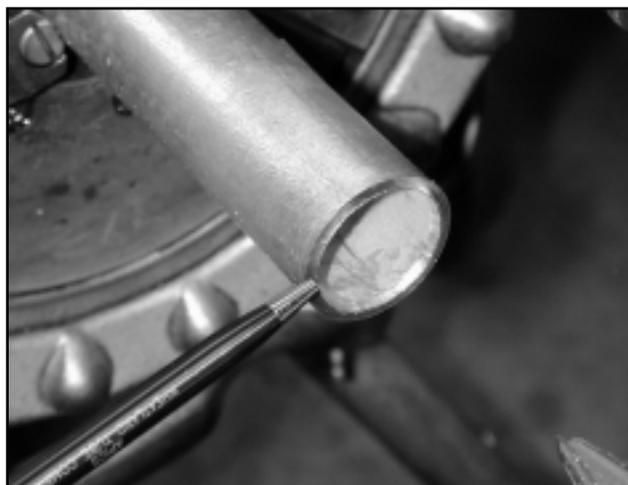
Figure 8: A minimal amount of pressure will remove the burr completely and eliminate possible flaring of the conduit end.
